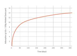
Adsorption rate is affected by part geometry. The plot shown is representative of typical performance at 25°C and 50% RH.
