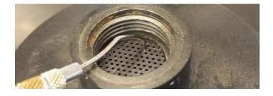
**4.** Once the perforated metal plate is removed, the desiccant can simply be dumped out. Note that desiccant is not normally considered hazardous and may be disposed of by normal waste disposal methods; however, refer to your local requirements for possible restrictions on disposal of spent desiccant.
