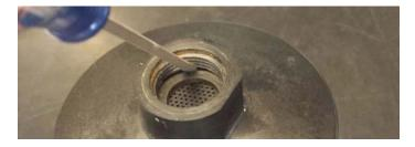
**3.** After removing the gasket, remove the perforated metal plate by "picking" it using a small pick as shown. A small paper clip will also work. The holes in the perforated metal plate are about .038" in diameter. The pick tool shown here has a small hook on the end of it. This allows the perforated metal plate to be easily lifted out.
