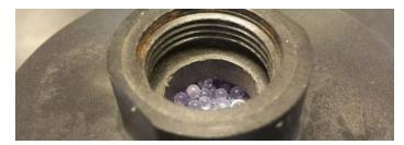
**5.** Refill the desiccator with fresh desiccant up to the level of the flat shown in the above photo. Gentle tapping and shaking of the desiccator during the filling process is advised to settle the desiccant as much as possible.
