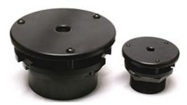
As magnetically-actuated one-way breather valves, AGM Ultra-High-Flow Valves provide protection for personnel and property during rapid decompression events involving containers that may otherwise explode. Reusable, the valve will automatically reseal after relieving excess pressure spikes. This comes as a benefit over competing products such as blow-out panels and membranes. The aluminum body construction provides durability while the nickel-plated
