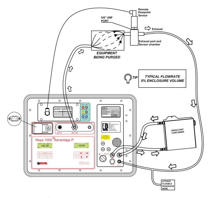
The preferred purging method when the enclosure is of a "light" construction, i.e. likely to deform under 1.5 psi internal pressure.
