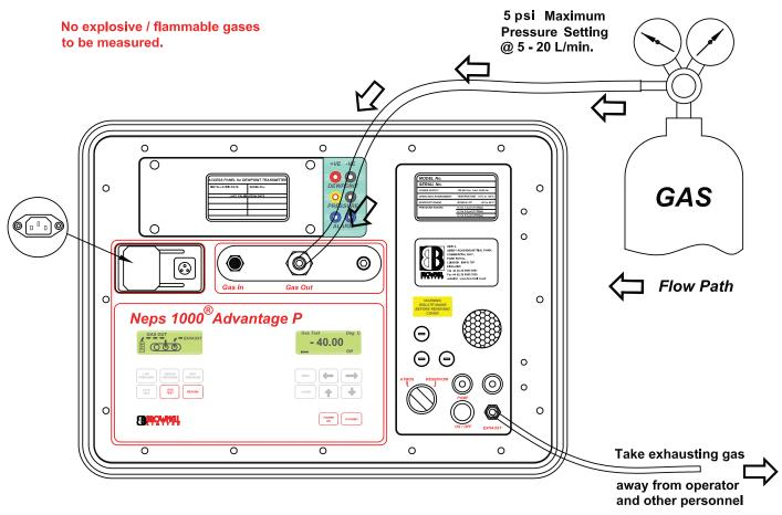
Select "Gas Test" - Duration of test is dependent on the gas being tested and its "wetness", i.e. the less moisture, the longer the test.
