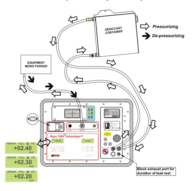
Select "Atmos" and with purging cycle underway, remove the flexible reservoir and block the exhaust tube and proceed with a normal purge cycle.
