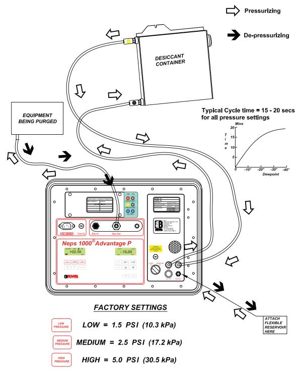
The structural strength of the enclosure being purged is the primary consideration when selecting the purge pressure. As the gas pressure rises, it "encourages" the contents of the enclosure to "give up" its moisture, so when the pre-set level is reached, the gas supply is shut off and the exhaust opened.
