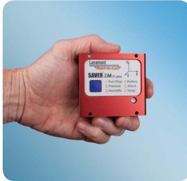
The SAVER™ 3M30 and 3M30 Plus are self-powered field data recorders with an internal tri-axial accelerometer. The 3M30 Plus is provided with temperature, humidity and atmospheric pressure sensors. The 3M30s are powered by a USB-rechargeable lithium ion battery, providing up to 30 days of continuous operation.
