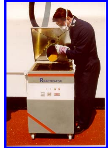
The 1005 Reactivator being filled with orange silica gel.
