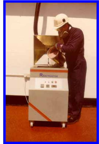
The Reactivator unit being filled with cobalt chloride impregnated silica gel
