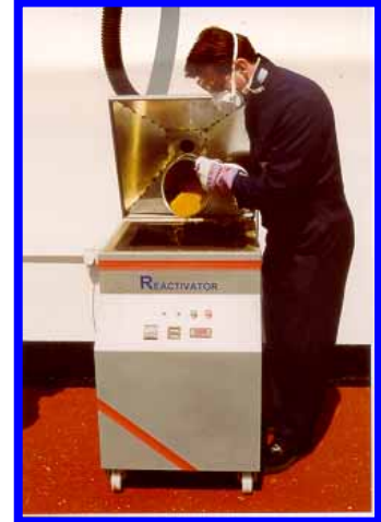
The 1005 Reactivator being filled with Envirogel.
